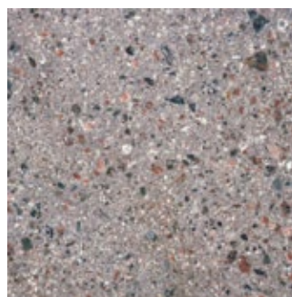
Examples of various concrete with pigmented cement and visible ballast
