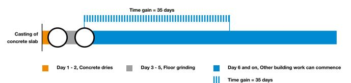
Allow the concrete slab to harden for 2 days. Then grind the slab smooth, removing the concrete skin which "opens" the concrete and allows the slab to dry faster. Once the grinding is finished, construction work can continue. As the slab is smooth from the grinding, no self-levelling compound is required. However, it must be watered and covered with plastic to avoid shrinkage cracks.
