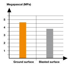
All the test results clearly show that the break occurs in the concrete and not in the joint between the concrete and the floor covering. The results also show that the shot blasted surface causes greater variations between the highest and lowest result (1.64 MPa), compared with the ground surface (0.7 MPa). This suggests that a shot blasted surface contains peaks with a worse C value and that the shot blasted surface risks containing micro-cracks.
